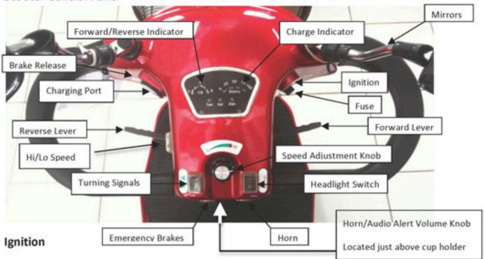
Place your keys in the ignition and turn **clockwise** one click to engage the motor. You will know the scooter is on once the LEDs light up on your control panel. To turn off your scooter, simply turn your key **counter-clockwise**.
