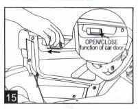
Red (yellow) button inside is for OPEN/CLOSE function of car door. When pushing the button backward and pulling the button upward to the top, the door will open (Please see Picture 15).
