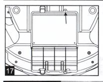
The cover plate at the front bottom of the car is designed for changing mainboard, loudspeaker or other accessories. When the accessories need to be changed, just unscrew the screw and open the cover plate, then you can see the mainboard cover(Please see Picture 17)
