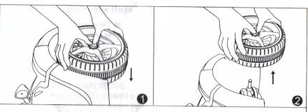
Steps of Wheel Installation: Set the wheel into the iron shaft straight until you hear a "click" sound and unable to pull the wheel back. It means the wheels are successfully installed. If you want to dismantle the wheel, pressing the wheel cover to remove the wheel.
