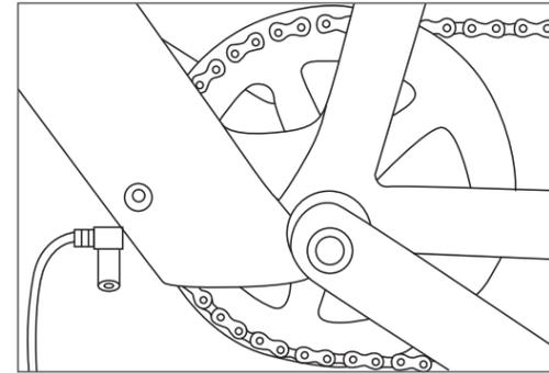
The charging port is located on the left bottom of the lower tube on the frame, covered by a rubber dust-free cover, uncover it, plug the charger into the port; cover the port again when charged.
