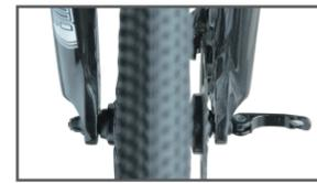
4. Insert the quick release lever on both sides of the front hub, and lock it.
