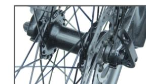
5. Adjust the switch of quick release lever and press to lock, complete the installation.
