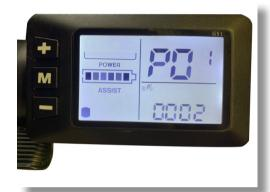
P01: Back light Display Brightness - level 1 is the darkest and level 3 is the brightest.
