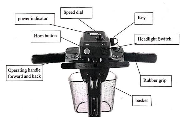
Electric door lock key to turn on /off the electric scooter.
