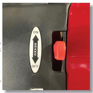
The unit must be on for the Parking Brake to work. And if the Parking brake is on you will not be able to drive forward.
