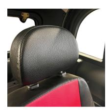
Look for the button under the left mounting rod (left as if you are sitting on it) and while holding that button in with your hand, raise or lower the head rest to your desired height.
