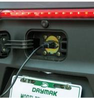
To access the charge port, take the keys and at the back of the unit unlock the charge port door. Inside you will find a plug. Lift up the cover and plug the charger into the socket.
