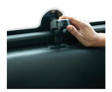
Then push the window open with your hand and while pushing the window open clamp the latch down to hold it in place.
