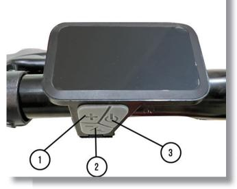
1) **Plus (+)** - Press this to increase the level of pedal assist , or to increase a setting value in the advanced menu (see next page). **Press and hold** this button to turn on the headlights.
