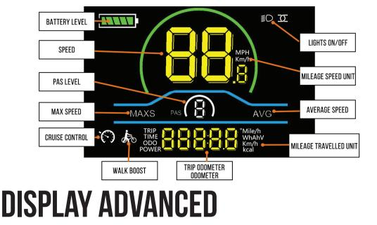
To access the advanced settings of your display press and hold the (+) and (-) buttons. To exit this menu press and hold the **Power Button** buttons again. Press the + or - on any flashing setting. To change the setting on any P Menu quick press the power button on any then press the plus or minus button to change it.
