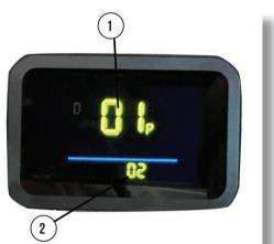
**P01**: Back light Display Brightness - level 1 is the darkest and level 3 is the brightest.
