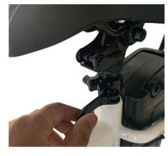
The Max S also comes with a seat raise feature that makes it so you can remove the battery while keeping the seat post in the frame.
